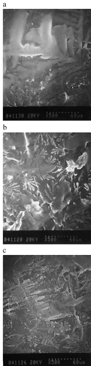
Fig. 5. Top SEM views of coated PG electrodes with the same magnification of 500 for (a) CMC films, (b) Hb-CMC films, and (c) Mb-CMC films.
